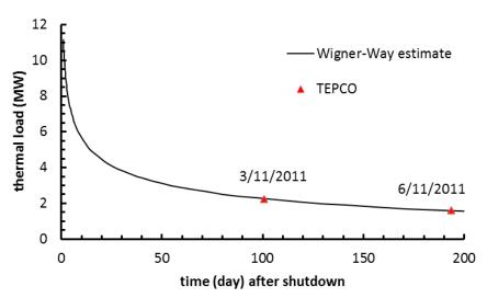
FIGURE 2B.5 Wigner-Way model of decay heat for the Unit 4 reactor core after reactor shutdown at the end of November 2010. Note: The data points are estimates by TEPCO based on the actual fuel inventory and a detailed model of the radionuclide decay.
