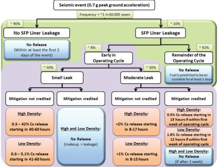
Note: The low-density pool has about 1/3 of Cs-137 inventory compared to high-density pool. Early in the operating cycle refers to early time after shutdown.
