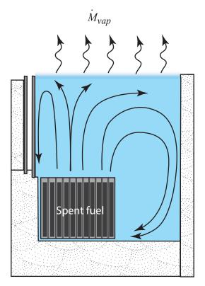
FIGURE 2B.1 Schematic of spent fuel pool showing the circulation pattern created by the buoyant plume of hot water above the spent fuel.
