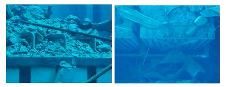
FIGURE 2.7 Images of debris in Unit 3 spent fuel pool on top of and beside the racks. *Left image:* Side view of the tops of the racks. Three fuel assembly handles are partially visible in the foreground of the image. *Right image:* Top view of the racks. SOURCE: TEPCO, used in NRA (2014, Figure 6.1).
