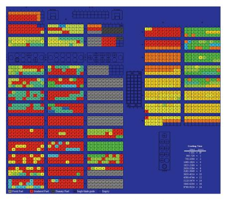
FIGURE 2.10 Fuel thermal loading in Unit 4 pool. Notes: The red squares indicate the hottest, most recently offloaded fuel assemblies. The grey squares indicate unirradiated (new) fuel assemblies. SOURCE: Wang et al. (2012, Figure 2). Copyright 2012 by the American Nuclear Society, La Grange Park, Illinois.
