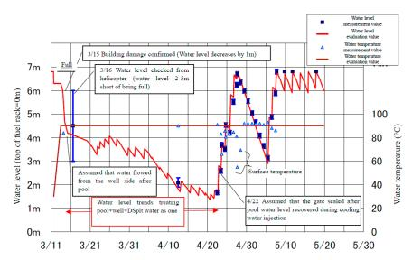
FIGURE 2.13 Water levels and temperatures in the Unit 4 spent fuel pool at the Fukushima Daiichi plant from March 11 to May 20, 2011. Notes: The squares and triangles are TEPCO-measured values of water level and temperature, respectively. The solid lines are TEPCO-modeled water levels and temperatures. SOURCE: TEPCO (2012a, Attachment 9-5, Figure 2).
