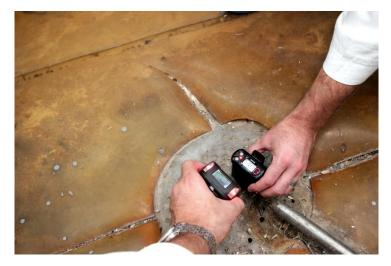
There are many drains and pipes where the gamma fields are over 3,800 uR/hr.
