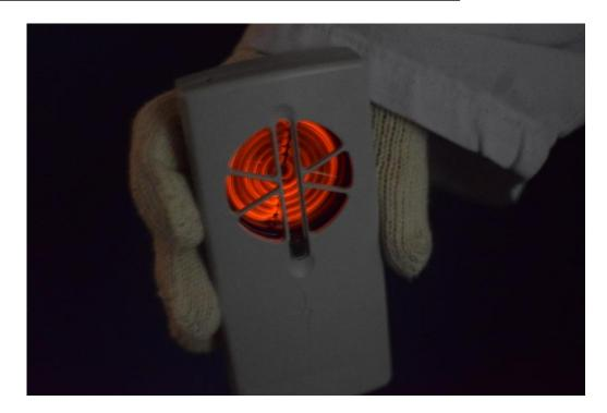
One of our group members brought a new detector that was being beta-tested for the manufacturer. The detector was specifically designed for better detection of beta contamination and operated better in the ventilation building than some of the other equipment in that regard. Some of the levels of contamination were so high that they caused the Geiger-Mueller tube in the device to glow red in the dimly lit rooms.
