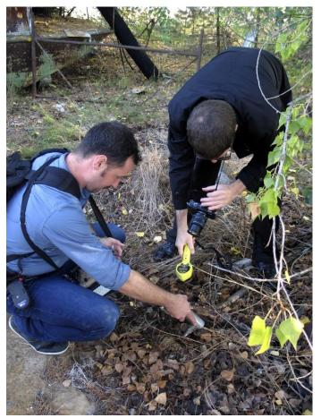
The gamma levels in the area of investigation were over 1,000,000 cpm at surface and peaked at over 3,460,000 cpm once the surface materials were removed and the dirt exposed.
