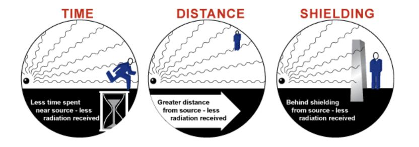
One of the radiation exposures of concern at Chernobyl is the gamma shine coming from the melted nuclear fuels in the Sarcophagus. The closer you get to the structure the higher the levels become, the more shielding between you and the structure – the lower the dose received.
