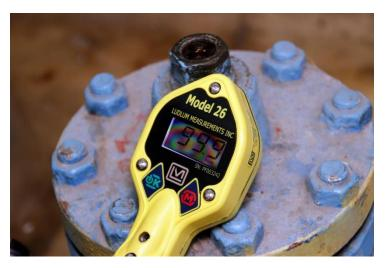
On top of some of the pipes and connections we were still able to detect large amounts of alpha and beta emitting radioactive materials which tended to max out the detectors capabilities.
