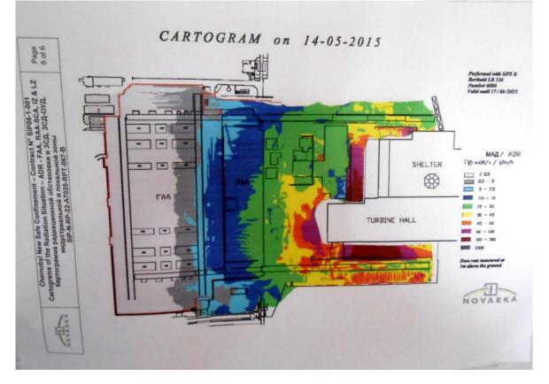
This is a map of the gamma shine levels around the Sarcophagus and "The Industrial Area" where the new confinement structure is being constructed.
