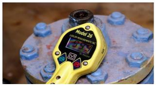
When conducting field surveys looking for contamination in the environment we used a Nal scintillation detector paired with a Ludlum Model 2350 Datalogging Survey Meter and a Ludlum Model 26 Integrated Pancake Frisker. Both of these units were calibrated to measure radioactive interactions in counts per minute.
