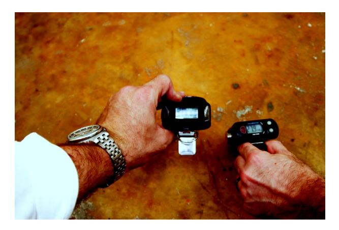
One of the most contaminated areas that we found in the maintenance corridors was a dimly lit stairwell with hotspots of contamination on the floor that contained gamma exposure rates over 48,260 uR/hr (48.26 mR/hr)).
