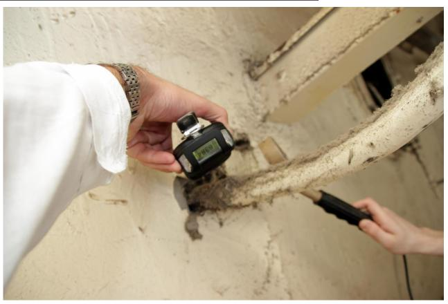
There is a continuing problem of contamination spreading and getting trapped in the dusts in the buildings. We continuously monitored the accumulating dust piles on top of pipes and rafters in the reactor buildings and main circulating pump rooms. We were able to identify areas with large piles of dust which maxed out the pancake detector with alpha and beta particles but where the gamma levels were no where near as high.
