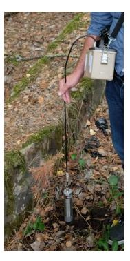
While traveling in the zone we utilized multiple methods of dose measurement. In addition to dosimetry provided by ChNPP I also took a CsI dosimeter which datalogs radiation levels and accumulates dose over time. The dosimeter tracks dose over time using the micro-Roentgen as the unit of measure. (1 uSv/hr = 100 uR/hr)
